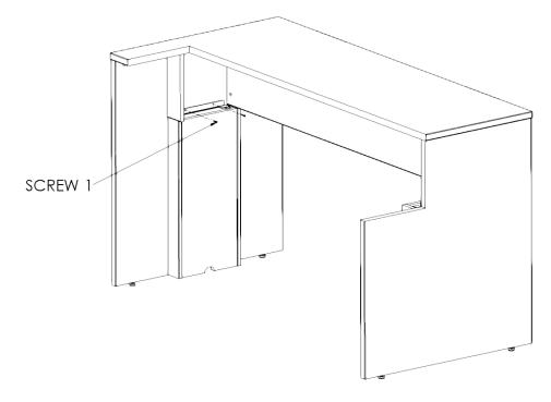
Install qty:2 screw 1 through top bracket into side panel to secure wire cover
